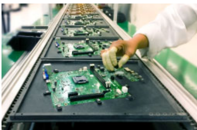
Transport boards for electronically sensitive devices
