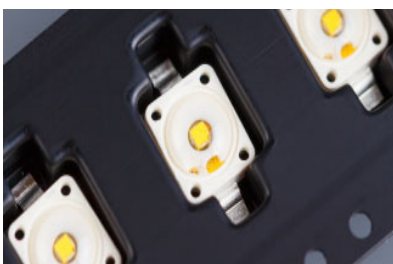
LEDs in conductive carrier tray
